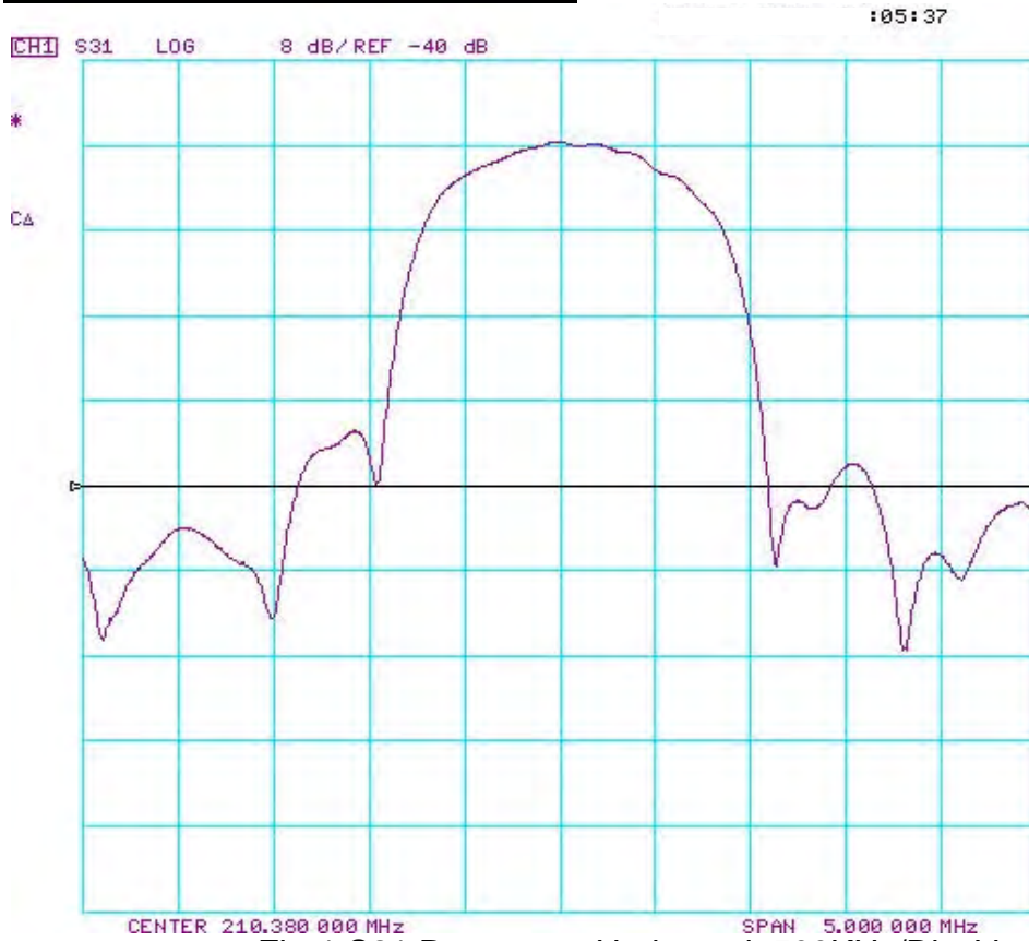
Fig-1 S21 Response Horizontal: 500KHz/Div. Vertical: 8dB/Div
