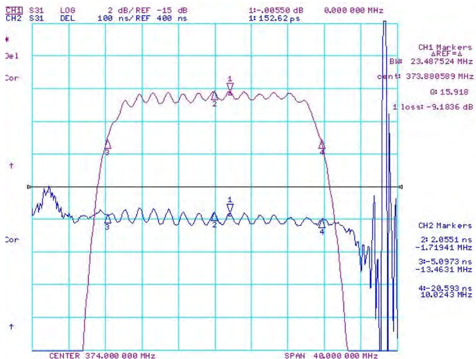
Fig-1 S21 Response Horizontal: 3MHz/Div Vertical: 5dB/Div, 100nS
