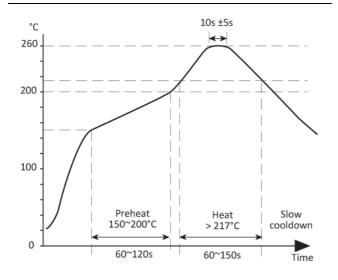
Lead free solderability limits:  $260^{\circ}$ C  $\pm 5^{\circ}$ C x  $10s \pm 5s$  x 2.
